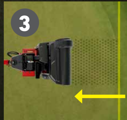
3 Coring head drops where aeration engaged
