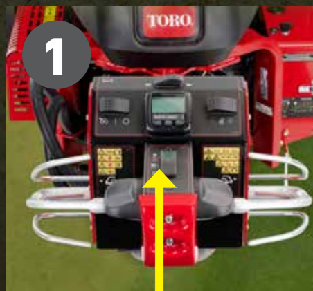
1 Set selector switch to Delayed Mode
